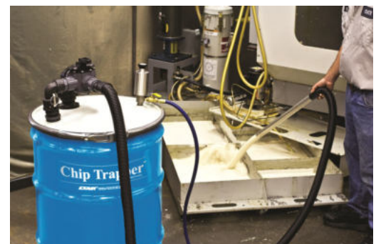
Emulsione filtrata da High Lift Chip Trapper
